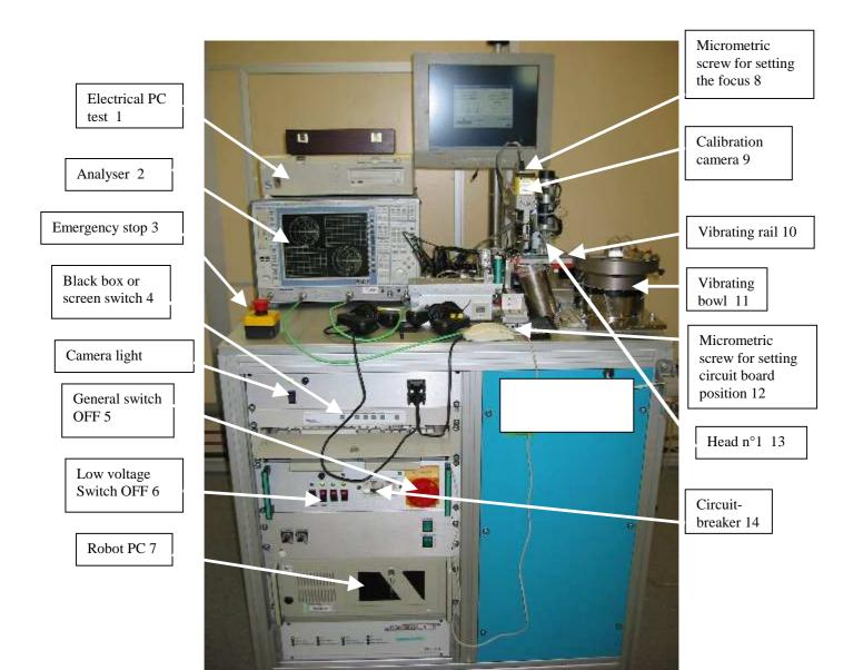
Position for placing doublesided components under test on the rail
