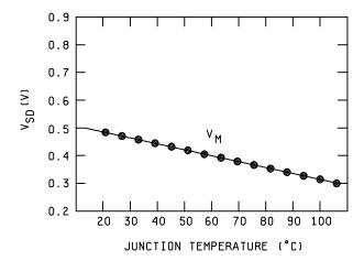
FIGURE 3161-5. Example curve of V<sub>SD</sub> versus T<sub>J</sub>.
