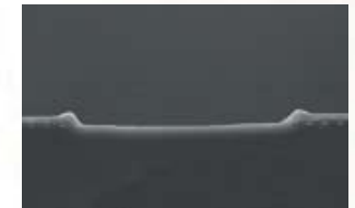
This SEM image shows a cross section of an IC wafer after laser scribing with NextStep . The image shows the clean trench left by the CO 2 laser
