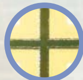
Scribe and dice process showing a well-confined dicing kerf within the laser kerf
