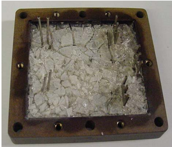
Figure 7. Module after 1500 hrs HTRB testing showing cracked RT-745S encapsulant.
